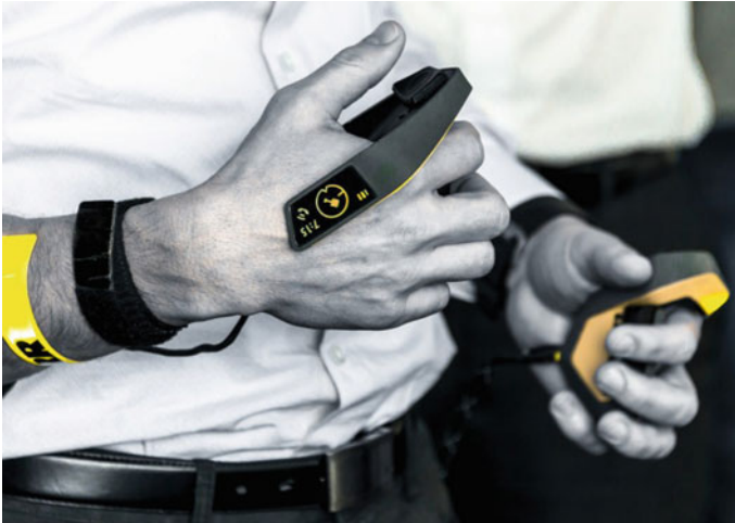
Fig. 14 Human-technology interaction with mobile cyber-physical systems: excavator controller designed by Emese Papp, Helge Wanta and Clemens Beyerlein for Liebherr
