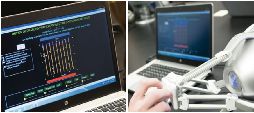
Fig. 13 A game-like scenario—user “grabs” a charged particle and moves it through an electromagnetic field, feeling the electromagnetic forces acting on it
