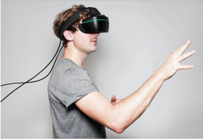
Fig. 15 (Cyber-physical) Technology demonstrator: VRieda VR/AR glasses using OLED micro displays designed by Philip Hart and Christian Hermeling for Fraunhofer FEP research institute
