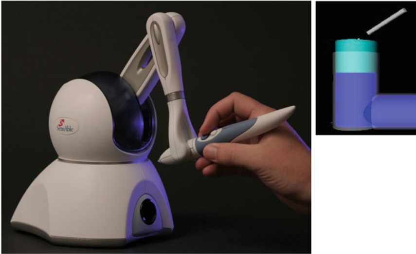
Fig. 9 Haptic interface-tactile feedback on pointer collisions with virtual objects
